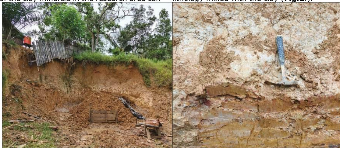
Fig.2. (left) The outcrop in the research area containing the soil that used as bricks (right) the close up view of the soil containing clay.
