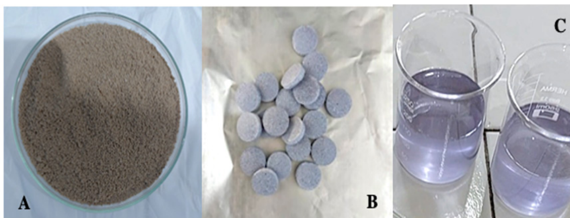
Figure 2. The result of bajakah root dried extract effervescent tablet optimum formula. There is co-processed excipient optimum ratio of 64: 36% [A], Bajakah root dried extract effervescent tablet [B], and solution of Bajakah root dried extract effervescent tablet [C]
