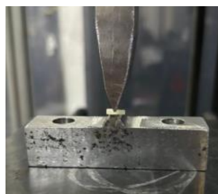
Figure 4. Three-point bending test performed on the specimens.
