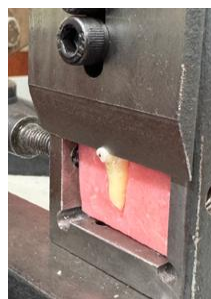
Figure 3. Shear strength test using a Universal Testing Machine
